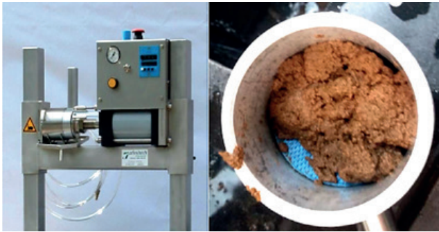
Figure 3. Photos of the press used in the tests and of the sludge after pressing
