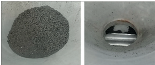
Figure 14. Photos of the sludge prepared with 15% moisture inside the hopper and the adhered residue, after transporting the material
