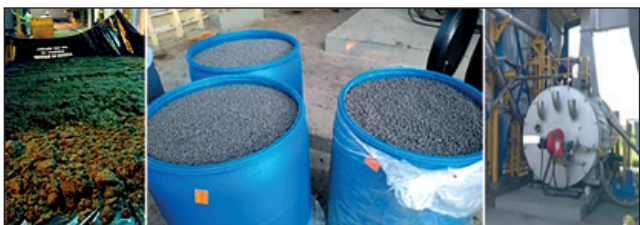
Figure 8. Photos of the sludge before and after the pilot test with a rotary dryer and the pilot dryer used
