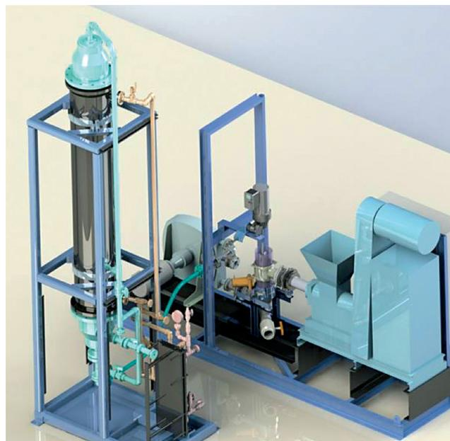
Figure 4: Design of pilot-scale continuous CNC reactor
